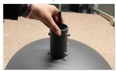
13. Mark the locations for drilling the hole 14. Drill two opposite holes into two opposite holes into the boom.
