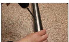
15. Lock with screws. Tighten allen screws with tightening torque of 8 Nm.
