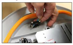
7. Connect the 2 core cable to the power supply (Class II.).
