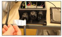
11. Tighten the cable glands and screw the cover back on.
