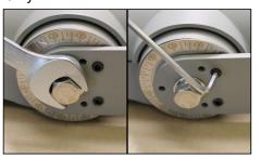
2a. Screw the auxiliary securing cable to the luminaire.
