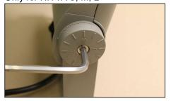
7b. Set the desired angle of the light fixture and tighten the locking screws. Tightening torque 10Nm.
