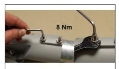
18. Losen two imbus srews to set an angle of the luminaire. Tightening torque of 8 Nm.
